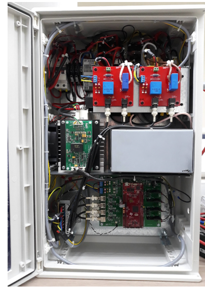
Figure 2: A microgrid DC-to-DC converter implemented for the DC microgrid in the IEPC labs.
